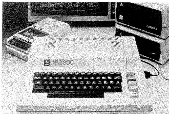
The Atari Computer has its BASIC interpreter stored on ROM in the form of a “cartridge” that can easily be inserted into the machine.
